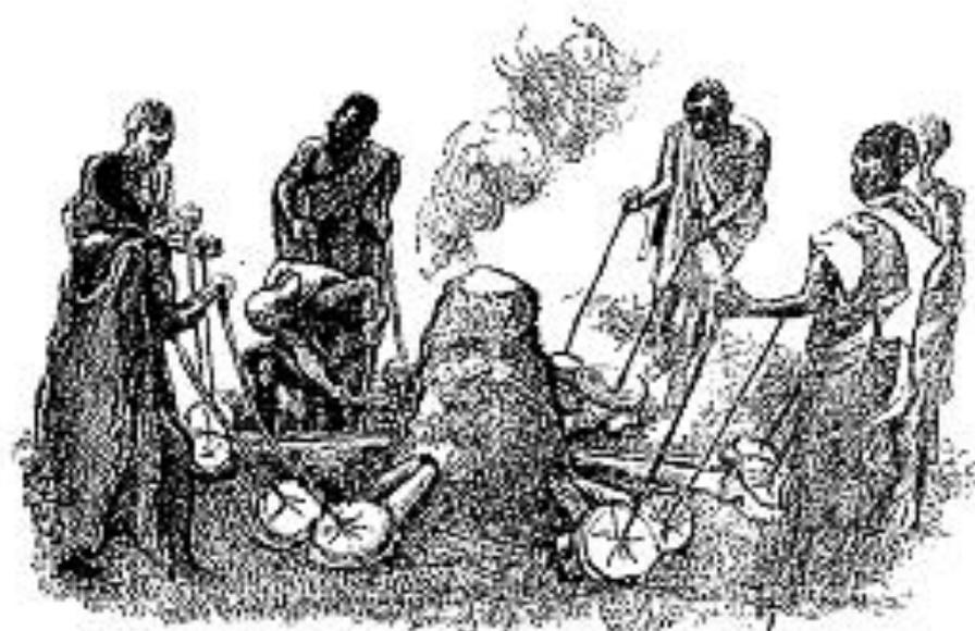
Bakiga blacksmiths smelting local iron ore. The temporary mud furnace is fed at the top with charcoal and the blast from the skin-covered bellows enters at the bottom
